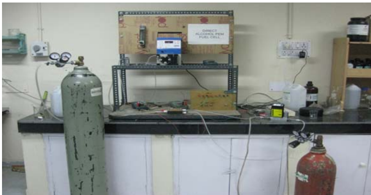
Figure 5. Experimental set-up for testing PEMFC at the Fuel Cell Laboratory, Indian Institute of Technology, New Delhi, India.
